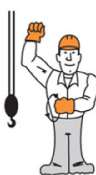
Crawler Crane Travel One Track
