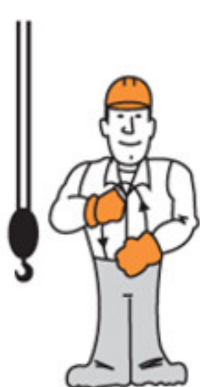
Crawler Crane Travel Both Tracks
