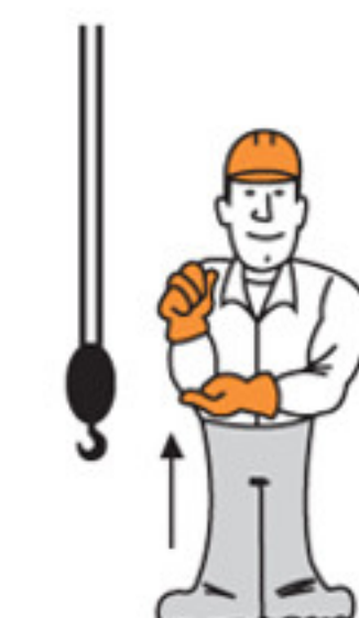
Use Auxiliary Hoist
